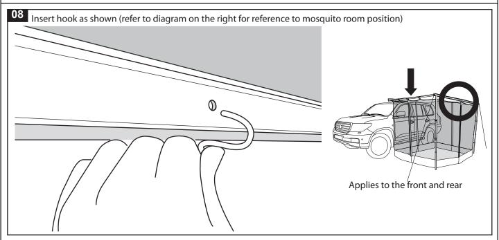
You can insert a peg through the metal hoop to secure the mosquito room in place (peg not supplied) or hook the ring under the spike in the leg
