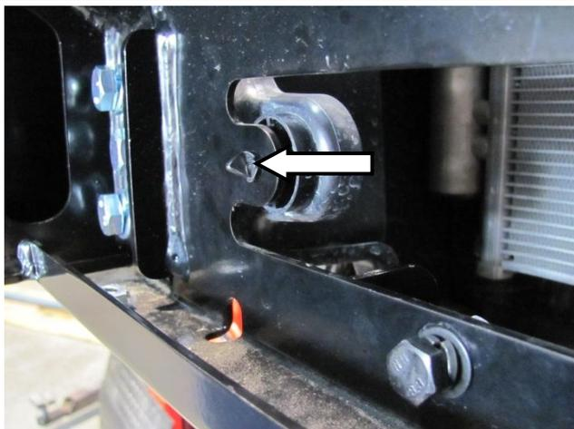
84. Using the original plastic clips re-fit the factory air deflector to the 2 holes in the mount bracket.
