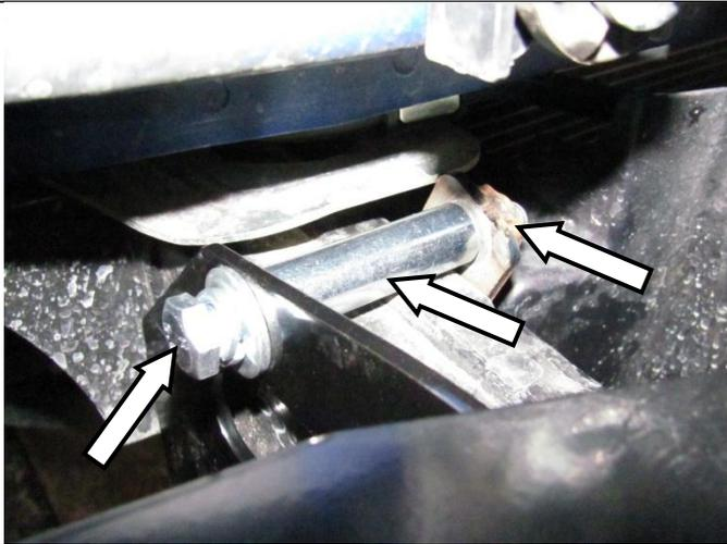
82. Secure the rear of the chassis braces to the chassis using 2 M10 x 80 bolts, 2 M10 spring washers and 2 M10 flat washers through 2 crush tubes into the nut plate assemblies on each side of the vehicle. Leave loose at this stage.
