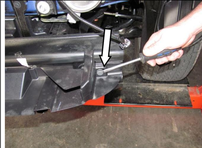
9. Remove the plastic panel attached to the front cross beam by removing the plastic clips. Discard the panel.
