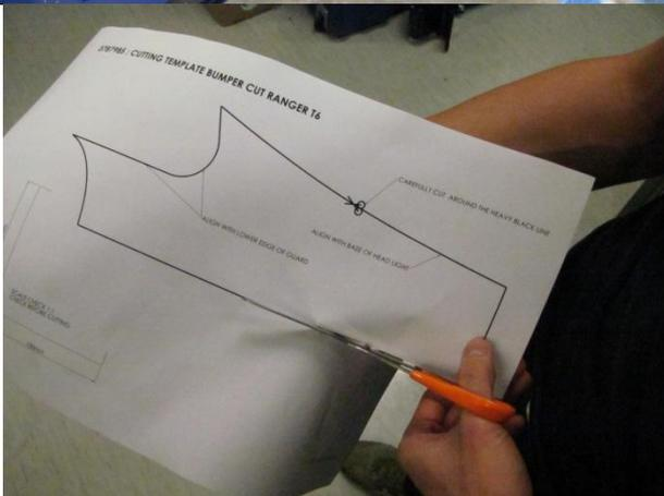
50. Using scissors carefully cut out the supplied paper template.
