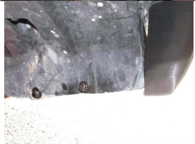
108. Mark and drill 2 Ø7mm holes through each of the inner guards in line with the cage nuts.
