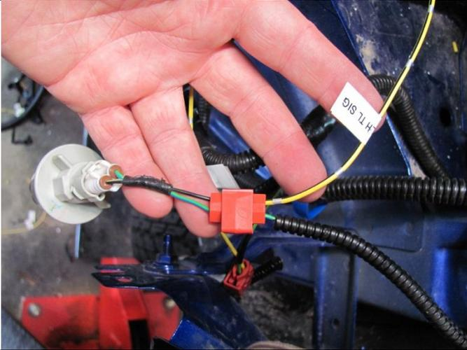
32. Starting on the LH side of the vehicle, scotch-lock the Clearance light signal wire of the loom (Blue / Black) to the OE positive clearance light wire (Green / Yellow).
