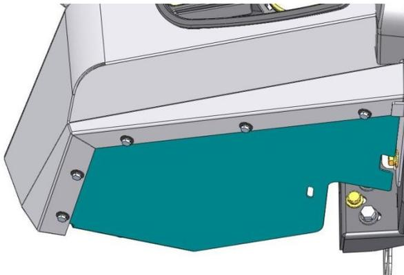
103. Fit the RH under wing panel to the RH wing as shown and attach using 5 M6 hex bolts, 5 M6 spring washers and 5 M6 flat washers.
