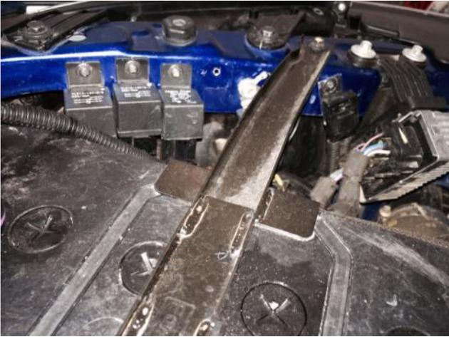
28. Using the tek-screws provided, attach the 3 relays to the panel directly behind the LH head light as shown.
