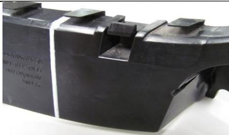
17. Use a saw suitable for cutting plastic and cut along the marker line.
