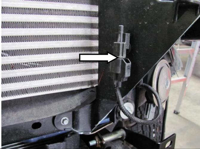
85. Using the pegs on the sensor removed in step 8 as a guide, Drill 2 Ø5.5mm holes in the LH air deflector so that the sensor can be fitted approximately 40mm forward of the rear edge of the air deflector as shown.
