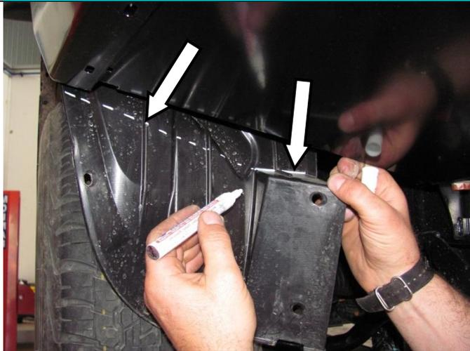
106. On the plastic OE inner guards, mark lines from the bottom corners of the bar wing tips down to the square corners in the inner guards. Continue the line along the horizontal corner.
