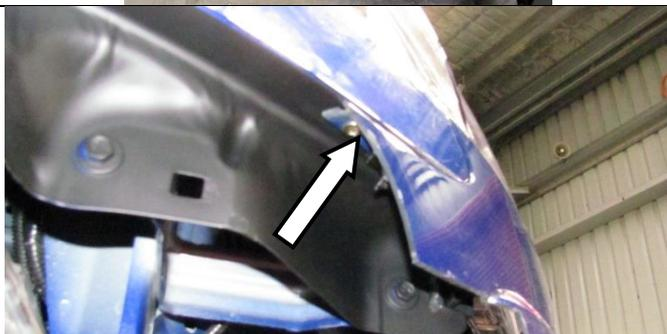
73. Drill an Ø2mm hole through each end corner of the bumper into the guard sheet metal.
