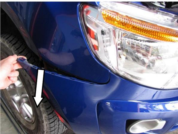
8. Starting on the RH side of the vehicle, carefully pull the rear most corner away from the vehicle un-clipping the bumper. With the assistance of another person remove the bumper from the vehicle and place in a safe place where it will not be damaged. Disconnect the sensor attached to the bumper and allow it to hang loose. If fog lights are fitted they will need to be disconnected.
