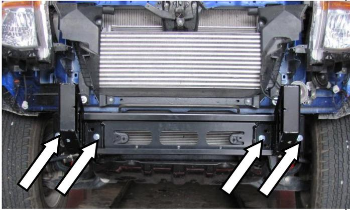
75. Attach the mount bracket to the chassis end plates using 4 M10 SEMS bolts into the captive nuts. Leave loose at this stage.
