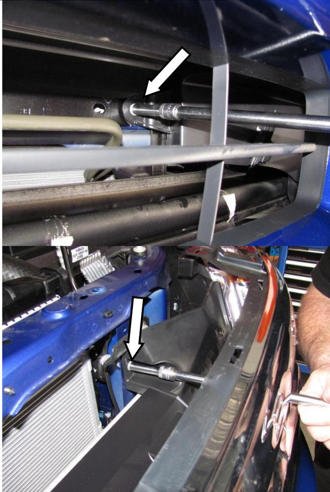
7. Using a socket extension, remove the screws holding the inner grille air deflectors to the vehicle. Place in a safe place.
