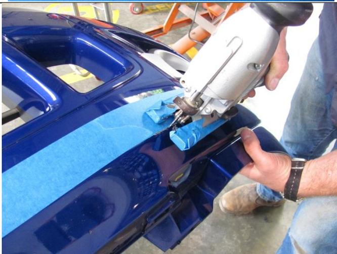
49. Using a jig saw or similar, carefully cut along the line made in the previous step.
