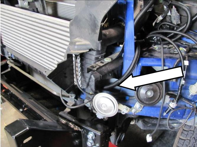
35. Route the remainder of the loom across the front of the vehicle along the cross beam that runs below the intercooler as shown.
