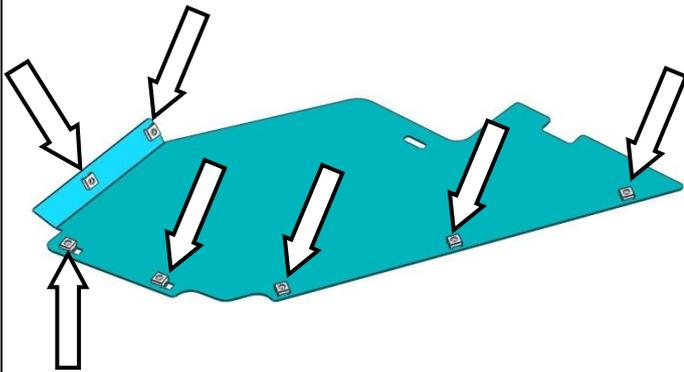
102. Fit 7 M6 cage nuts to each of the under wing panels as shown.
