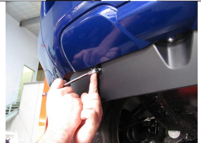
5. Remove all the fasteners securing the bottom of the bumper to the vehicle.
