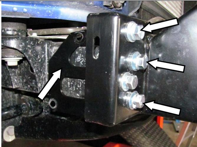
76. Place the right hand chassis brace onto the back of the chassis face plate and loosely attach it to the mount bracket using 3 M12 bolts, 3 M12 spring washers and 3 M12 flat washers and 3 M12 Flange nuts.
