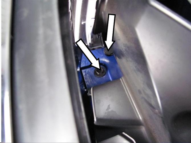
6. Undo and remove the screws and plastic clips behind the grille near the lower inner edge of the head lights.
