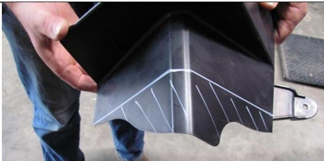
59. Mark the RH air deflector removed in step 46 as shown using the bottom edge of the lower mounting lug as a starting point across to the bottom corner of the opposite edge.
