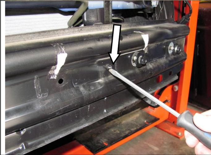
10. Use a screw driver to push the 2 plastic clips inward from the front cross beam. Do not remove the clips as they will be used later.
