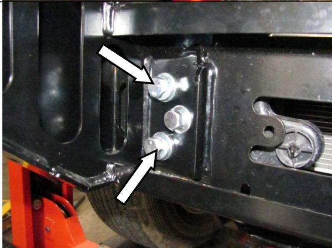
78. Place 2 M12 bolts, 2 M12 spring washers and 2 M12 flat washers and 2 M12 Flange nuts into the 2 holes on the inboard side of each chassis face plate. Leave loose at this stage.
