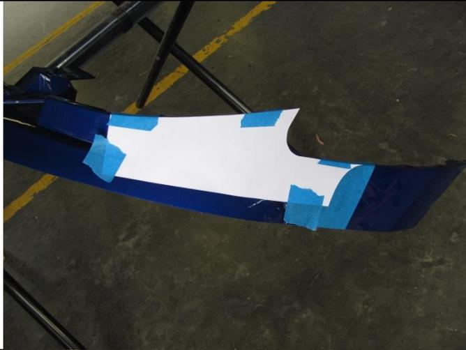
51. Attach the template to the bumper as shown using masking tape.
