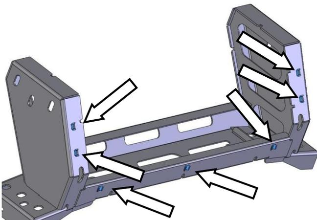
80. Fit 7 M8 cage nuts into the mount bracket from the inside.
