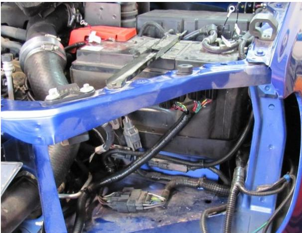
29. Route the battery positive and the battery negative wires to the relevant sides of the vehicles battery. Do not attach at this stage.
