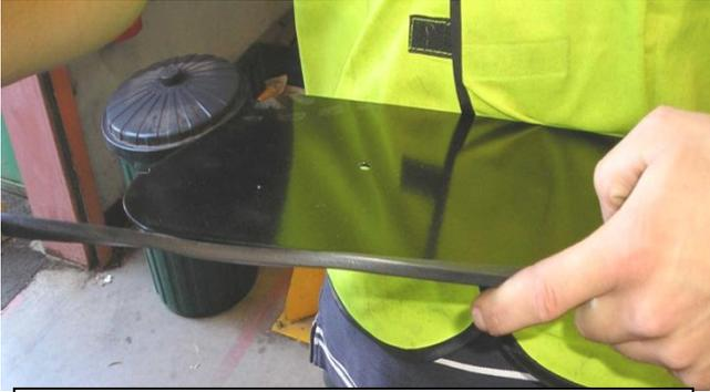
Applying trim rubber, note the join is at middle of the rear of the plate or long side.
