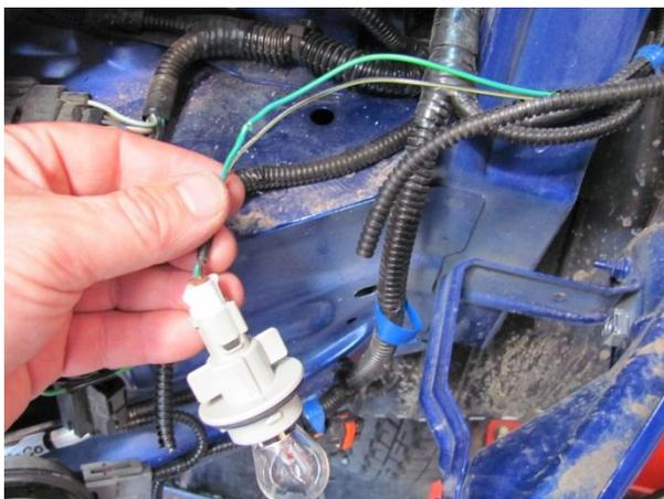
30. On each side of the vehicle, carefully cut back the protective tubing from the turn light globes wiring being careful not to damage the wires inside.
