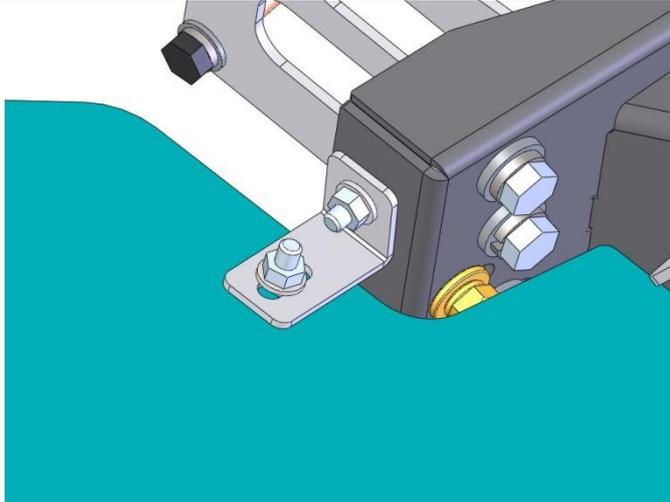
105. On each side of the bar attach the under wing panel to the mount bracket with the wing panel bracket using 2 M8 hex bolts, 2 M8 spring washers, 2 M8 flat washers and 2 M8 flange nuts.
