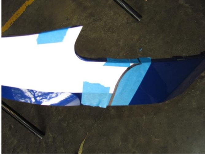
53. Using a marker pen, carefully trace a line along the rear most edge of the template continuing down the cut edge of the bumper.
