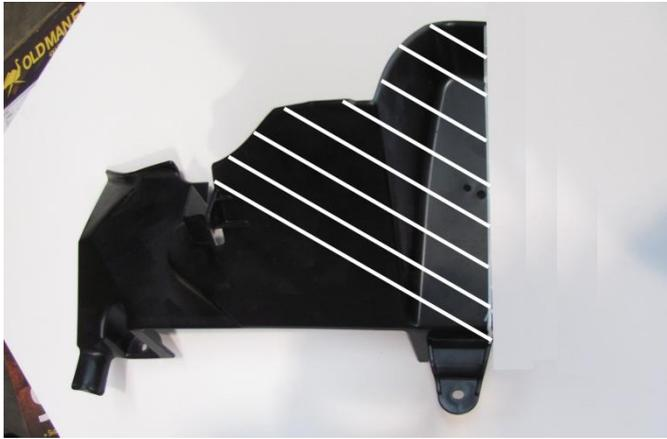
63. On both the RH and LH air deflectors, mark a line from the bottom corner of the lower mounting lug up to the forward / bottom edge of the bumper mounting lug as shown.
