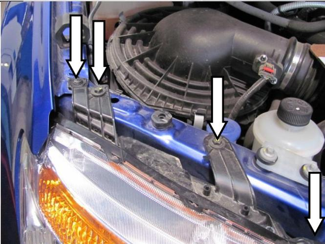
26. Carefully remove the head light assemblies from the vehicle, carefully unclipping the main head light globe plugs and completely removing both the turn tight globes and left hand side clearance light globe.
