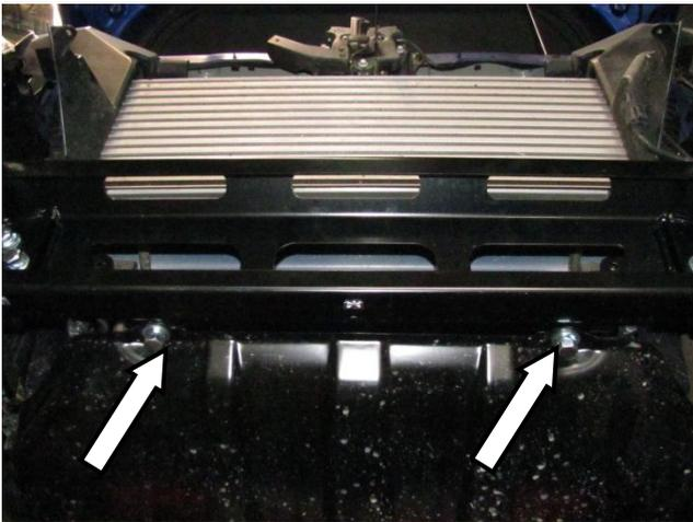
83. Re fit the OE stone shield to the bracket fitted in step 81 using 2 M10 SEMS bolts and 2 M10 flange nuts.
