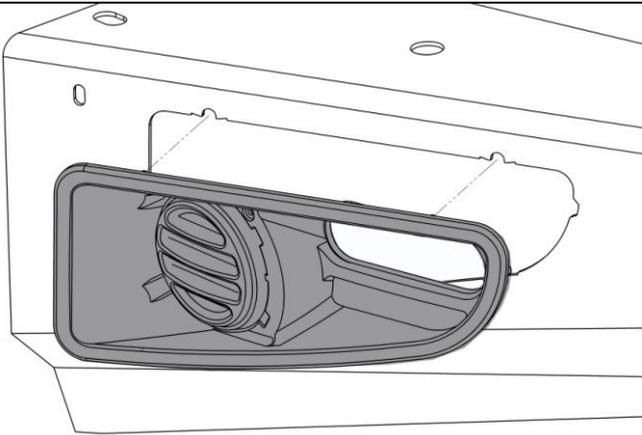
100. Assemble and install combination light surrounds (p/n 3163015) as per instructions no. 3786421 supplied with surround kit. Note: Optional fog lamps can be installed at this point as per fitting instruction no. 3783315 supplied with fog lamp kit no. 6821201.
