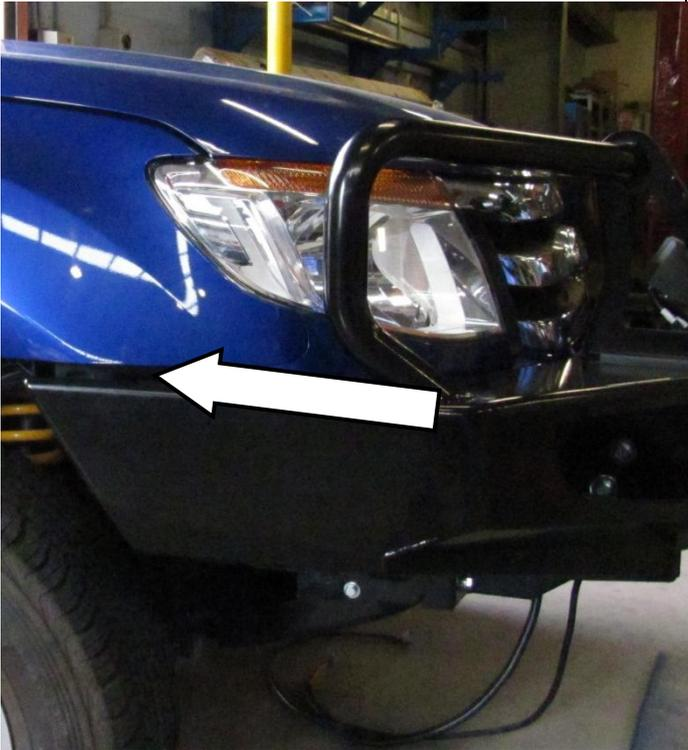
92. Position the bar so that it is level and there is a gap between the top face of the wings and the bottom edge of the guards of 18-22mm and the wing tips are aligned with the edge of the wheel arch.
