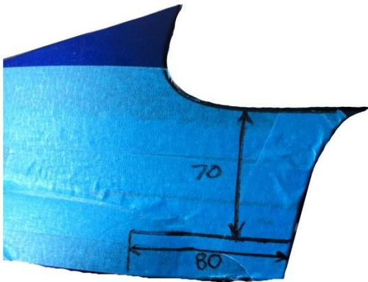
56. Mark 2 lines on each side of the bumper 70mm down from the edge that mates with the vehicles guard and 80mm from the rear most edge as shown.
