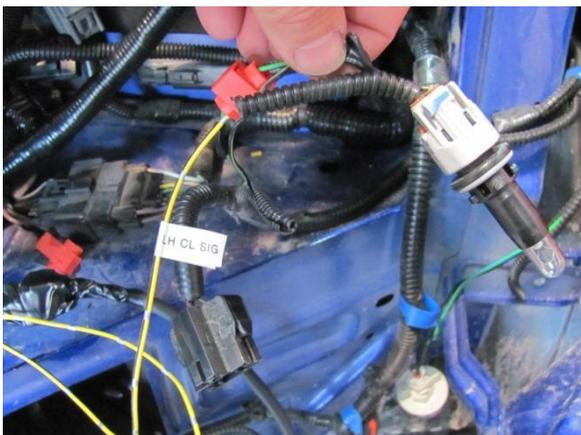
36. On the RH side of the vehicle, scotch-lock the Right Hand turn light signal wire (Yellow / Black) to the OE positive turn light wire (Blue / Yellow)
