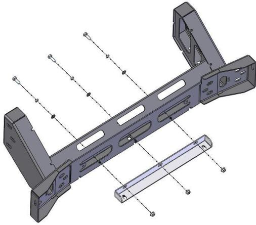
81. Attach the OE stone shield bracket to the chassis mount using 3 M8 x 25 black bolts, 3 M8 black flat washers, 3 M8 black spring washers and 3 M8 flange nuts. Leave loose at this stage.
