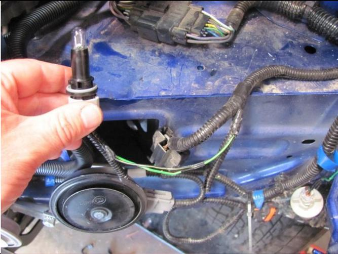
31. On the left side of the vehicle, carefully cut back the protective tubing from the clearance light globe wiring being careful not to damage the wires inside.
