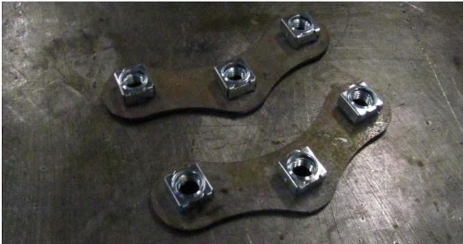
89. Fit 3 M12 cage nuts to each of the cage nut plates.
