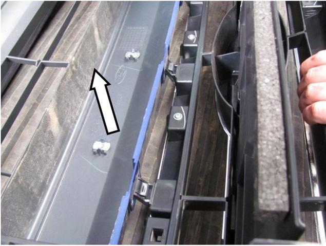
13. Carefully unclip the grille from the bumper and place in a safe place.
