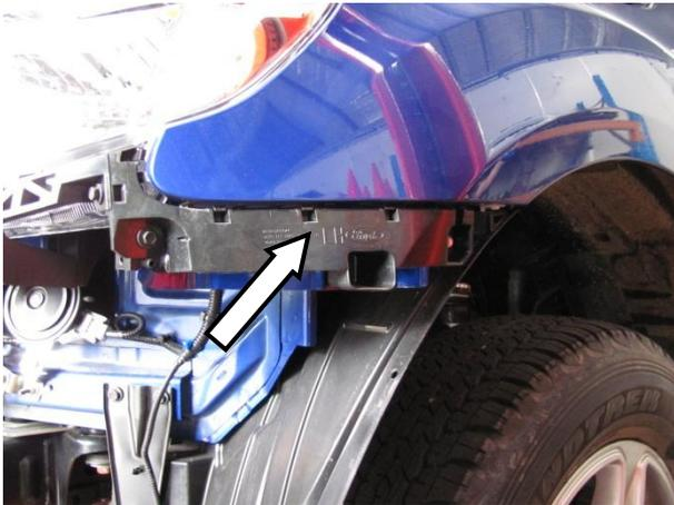
14. Remove the RH and LH bumper retention blocks from either side of the vehicle and place in a safe place.
