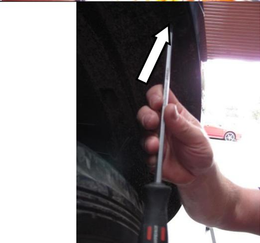
4. Remove all the bumper fasteners along the inside edge of the wheel arches.
