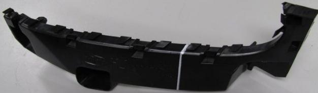
16. Starting with the RH bumper retention block removed in step 18, mark as shown using a white marker pen. Note the position of the marking in relation to the lugs on the top edge of the block.
