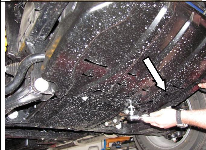
12. Remove the factory under panel and place in a safe place. Do not completely remove the rear bolts. Leave loose.
