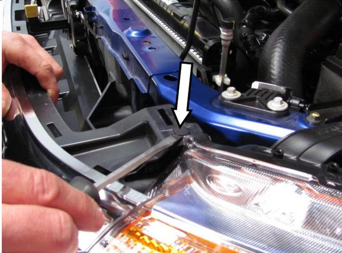
3. Remove the plastic clips from the top / rear corners of the grille. Place clips in a safe place.
