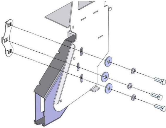
91. Attach the bar to the mount bracket using 6 M12 bolts, 6 M12 spring washers and 6 large diameter M12 flat washers, into the nut plates which are placed inside the box upright sections of the mount bracket. Leave loose at this stage.
