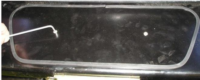
113. Fit the panel to the top of the bull bar as shown using M6 pan head stainless steel screws, M6 flat ss washers and M6 flange nuts.
