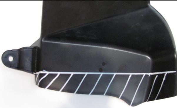
61. Mark the LH air deflector removed in step 46 as shown using the bottom edge of the lower mounting lug as a starting point, marking a line perpendicular to the vertical edge below the lug.
