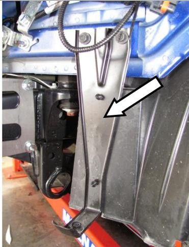
15. Remove and discard the inner guard support brackets from both sides of the vehicle.
