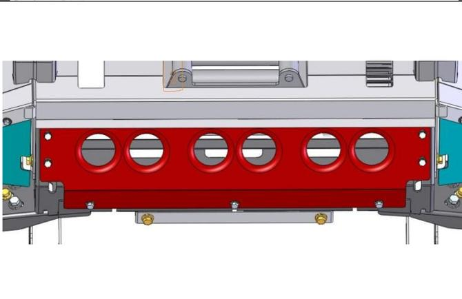
110. Attach the centre stone shield to the mount bracket using 7 M8 hex bolts, 7 M8 spring washers and 7 M8 flat washers into the cage nuts fitted in step 79.
