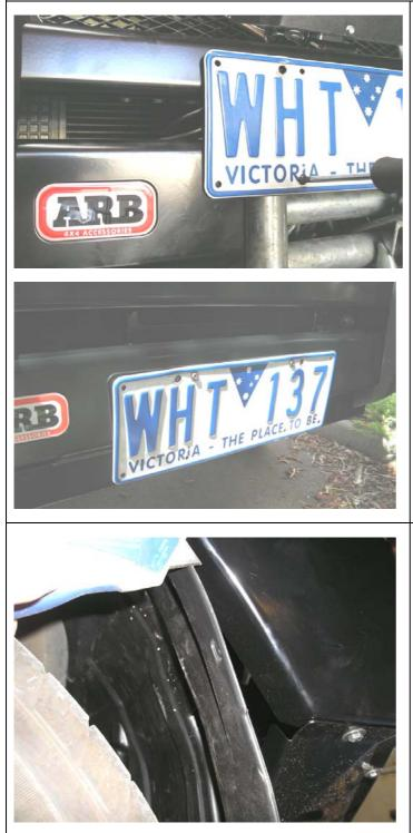
84. The licence plate can now be attached to the bull bar. Insert the two plastic square plugs supplied into the two square holes in the face of the bull bar (note slot allows for adjustable number plate hole pitch, ensure grommet flanges fit over the narrow width of the slot to engage correctly).
