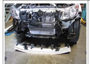
27. Remove reinforcing beam at mounts to chassis by undoing the M10 fine thread bolts. Set beam aside, it will not be reused
