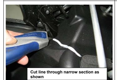
28. Mark a cutting line as shown then cut plastic air deflectors, both sides so lower portion is removed to clear bull bar mounts.
