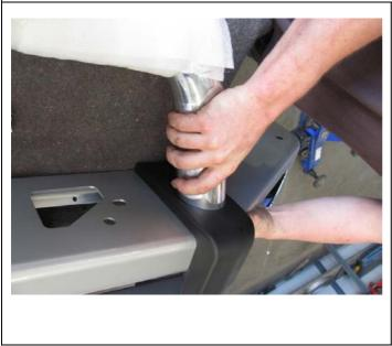
49. If fitting frame *P# 5121010*, locate frame as shown and then from below inside wings, secure with M12 x 50 bolts and washer sets
