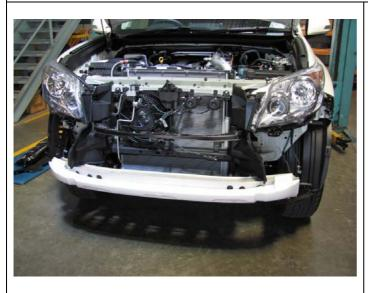
26. Remove reinforcing beam foam pad, then remove the beam, *refer next step*.
