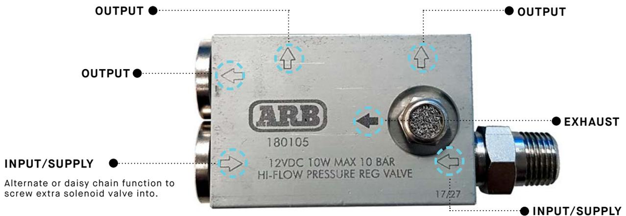
1. The LINX PRV must be connected to a compressed air source that has a higher minimum output pressure than the maximum required of any connected accessory. The LINX PRV comes with a 1/8 BSPT nipple pre-installed. If desired this can be relocated to the input port on the opposite side by removing the threaded plug.
