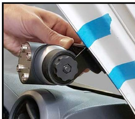
**STEP FOUR:** Turn the A-pillar Bracket upside down, then hold it on the outer side of the pinch weld seam to mark the position of the holes to drill.
