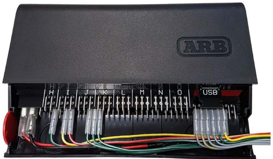
**NOTE:** Pins C3, C4 & C5 have been connected to 180422 (LINX Relay Harness) in the above image.
