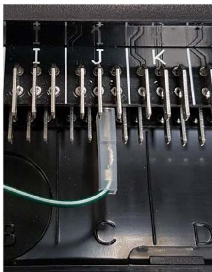
Connect the accessory wire to digital output terminal C3:
