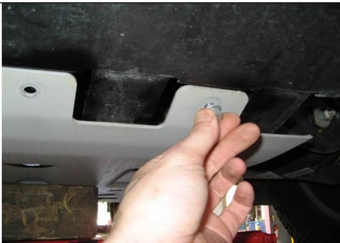
7. Place front panel in position and secure front using 3 x M8 button head cap screws, spring washers and flat washers. Leave finger tight.
