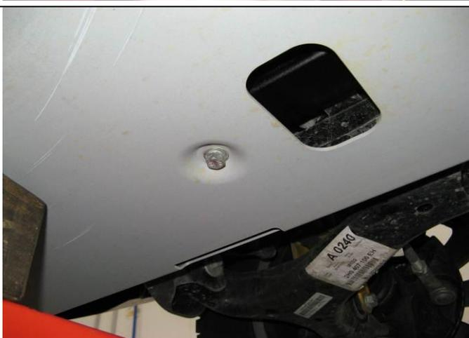
8. Secure rear of front panel using 2 x M8 x 25 bolts, spring washers, flat washers and M8 flange nuts. Leave finger tight.
