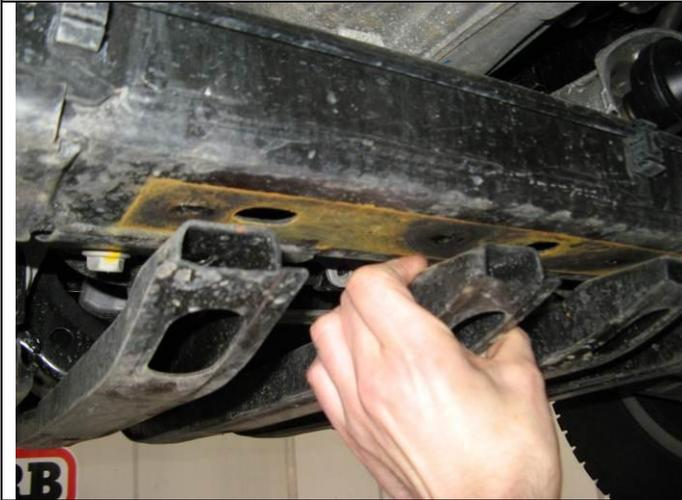
2. Remove rear mounting bolts from front skid rails. Pull away from chassis slightly. This must be done to gain clearance to fit front bracket.
