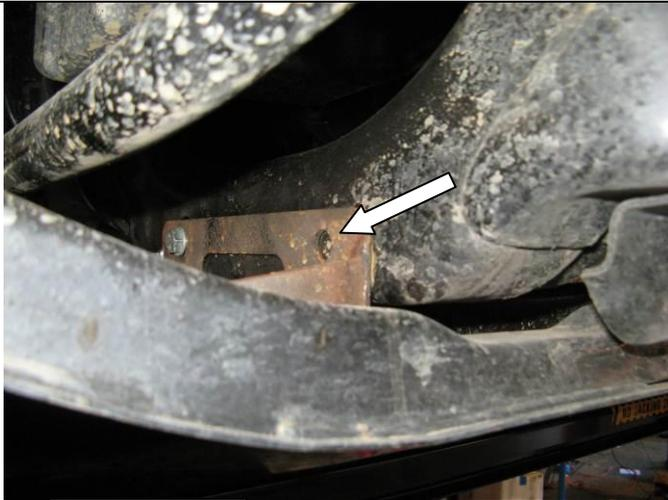
5. Once bracket is in correct position mark other hole using a white marker pen. Remove bracket and drill hole using 9mm drill bit. Re-fit bracket when done and secure with an extra cage nut plate, M8 cage nut, M8 x 25 bolt, spring washer and flat washer. Adjust bracket once again as per step 4.
