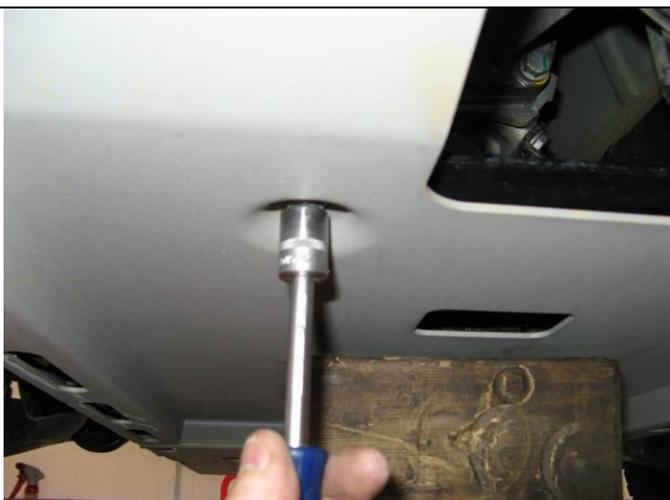
12. Secure rear of panel using 2 x M8 x 25 bolts, spring washers, flat washers and M8 flange nuts. Once all is fitted correctly tighten all bolts.
