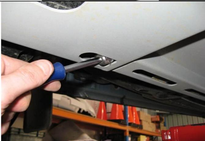
11. Lift transmission panel into place and secure front using 3 x M8 x 25 bolts, spring washers and flat washers. Leave finger tight.
