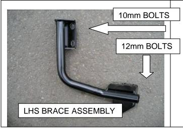
29. After fitting impact absorbers to vehicle, the brace assembly is next to be fitted.
