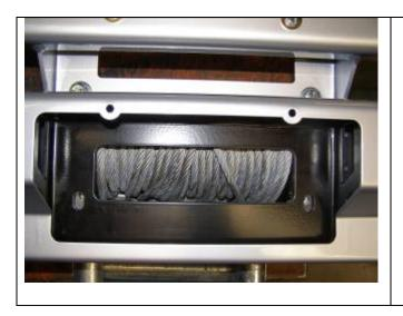
56. Lower bar down over winch, line up top holes first and secure these only using 3/8" hardware (1 ½" x 3/8" bolts) with flat and spring washers (finger tighten only)
