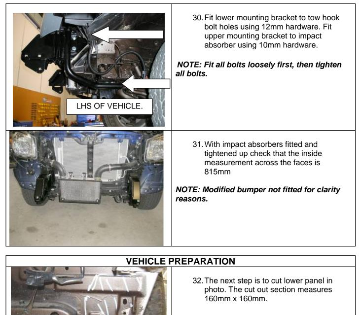
NOTE: This is to give ground clearance and aesthetics to the vehicle with mounted bull bar. Not required if fitting wing panels. NOTE: ( Completion of this step is decided by the owner of the vehicle, see note on Page 1 )
