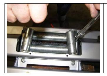
60. If circlips were removed, refit rollers and circlips after tightening bolts.
