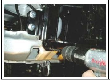
61. Drill Dia 10.0 pinning hole in lower flange of mount bracket into the vehicle crossmember
