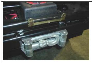
75. Fit number plate bracket as shown using M6 hardware.
