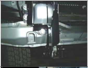
62. Fit M10 SEMS bolt and load flange nut from inside cross member then do up tight.
