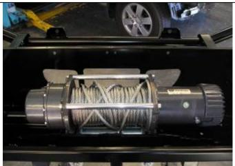
66. Insert winch into position as shown
