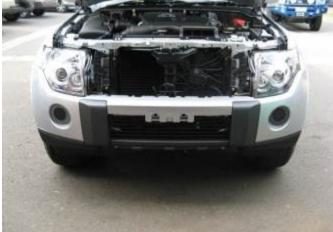
18. Place bumper back on vehicle including securing wing area of bumper into retaining clips.
