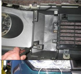
16. Remove the two buffer blocks from the bumper. Fixing screws are accessed from rear of bumper as shown.
