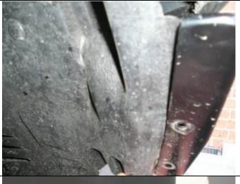
88. Tuck fender liner into inside rear of wing flange.
