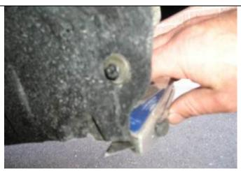
91. Carefully, using a sharp knife or hacksaw trim off the fender liner co-incidental with the lower edge of the cross beam.
