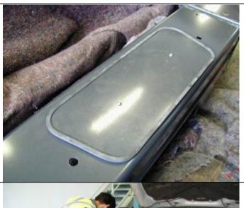
81. Fit panel to top face on bull bar using 2 x M6 dome head stainless steel screws, flange nuts and stainless steel flat washers.
