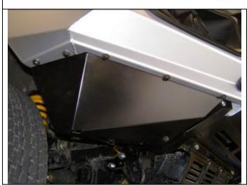
99. Fit the M6 cage nuts to the under wing pans and fit to the underneath of each wing using M6 x 16 Hex bolts, M6 Washers and M6 Spring Washers.
