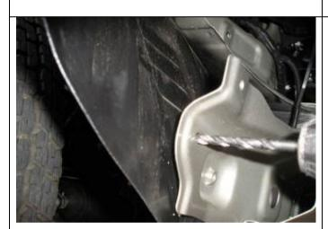
90. Drill hole in fender liner and cross beam as shown and secure liner with M6 black bolts, washers and flange nuts.
