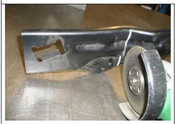
29. Using a jig saw or angle grinder with cutting wheel, cut along the line.
