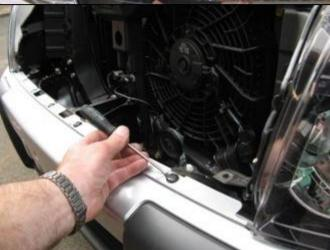
7. Remove upper bumper retaining scrivets.
