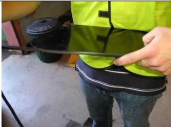
80. Apply rubber mold to edge of winch hole cover panel and trim off excess.
