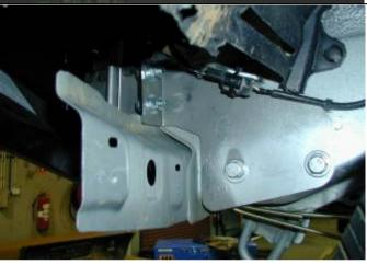
63. Reclip electrical loom connector into new bracket flange both sides of vehicle.
