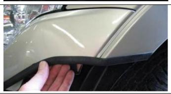
42. Fit the pinch weld to cut edge both sides.
