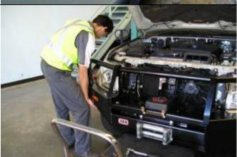
82. Support bull bar on lift device if available or with the help of one or more assistants lift the bull bar into position on the mount brackets.
