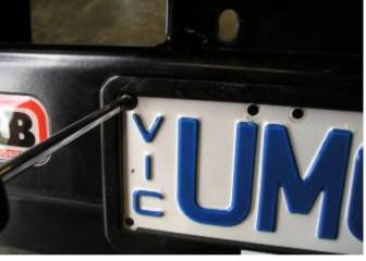
79. Fit number plate using black dome head screws inserted into grommets.
