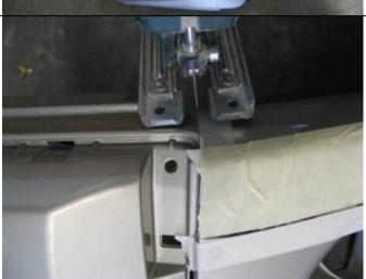
25. Using a jig saw or similar suitable cutting device, cut along the line. The cut through the top of the bumper is aligned with the edge of the buffer recess as shown.
