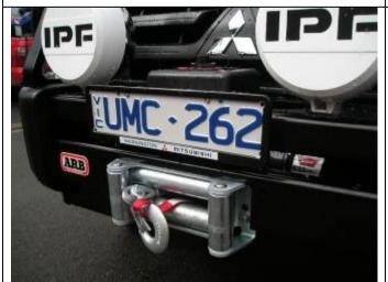
76. Fit number plate located as shown using M6 hardware.
