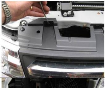
6. Remove scrivets securing grille across the top and pull grille upward to release lower clips.
