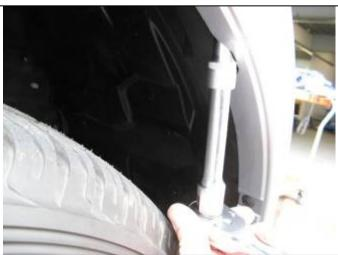
5. Undo vertical screws securing bumper to fender
