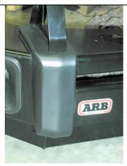
77. Insert the side buffers through the holes and fix using the M6 flange nuts.
