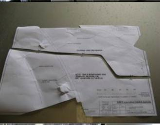
20. Remove template from vehicle and cut along designated cut line, also if required in various other areas to assist aligning to vehicle, as shown.
