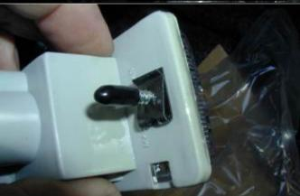
96. Remove indicators from cartons and then remove screws and speed nuts from each light. These fasteners are not to be reused – new screws are supplied in the fitting kit
