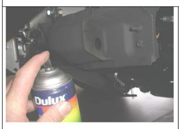
92. Using a black spray pack, paint the exposed color coded area of the cross beam so it does not show.
