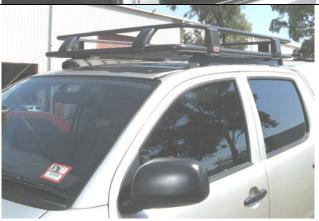
22. With the assistance of another person, lift the roof rack onto the vehicle and position evenly.
