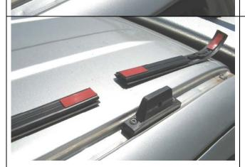
20. The fitting kit includes two pieces of double-sided tape to be cut into equal lengths of roughly 50mm lengths (12 pieces). Apply tape to each end of the roof trim pieces and stick the roof trim back in place.
