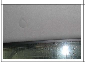
2. Remove the plugs located around the periphery of the ceiling. They are located at the front at the driver's side, the rear of the ceiling at the right and left hand sides of the vehicle and above the rear windscreen.
