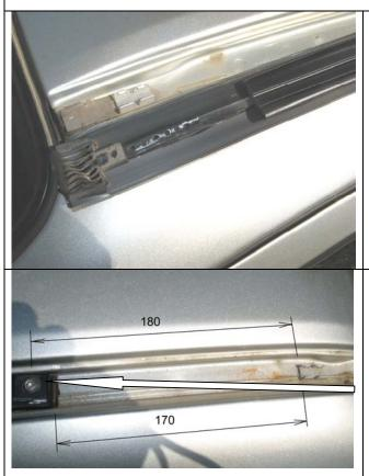
8. Remove the exterior roof trim from both sides of the vehicle. Take care not to bend the trim, as it will be reused.
