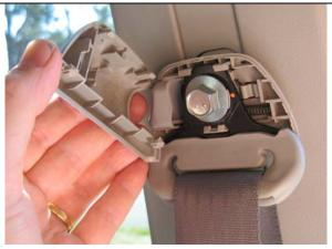
5. Remove the front and rear top seatbelt mounts.
