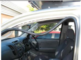
4. Pull down the door seals so the interior trim can be removed.
