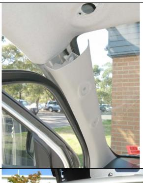
6. Remove the plastic trim from the front, middle and rear pillars on each side of the vehicle. They can simply be pulled away to be released from their mounting clips.
