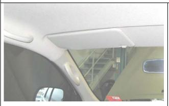
1. Remove the sun visors. Remove the two grab handles front the front pillars and the grab handle front the ceiling on the passenger side of the vehicle.
