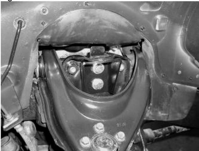
Position the support bracket and captive nut plate on the original shock absorber mount.
