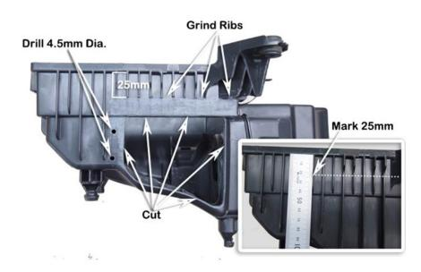
Using a body saw or die grinder remove the ribs as shown.
