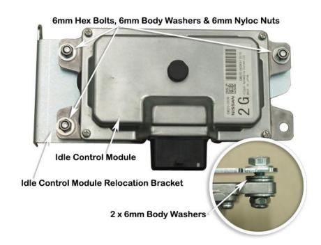
Remove the module from the inner guard panel shown, retain 6mm hex bolt.
