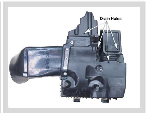
132 Install the air cleaner base and hose assembly into the vehicle. Hint: squash the end of the hose whilst installing through the hole in the inner guard.
