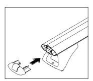
When the leg assemblies are fitted to the vehicle, then tighten M6 bolts to 3-4Nm. Do not over tighten. Measure slot length (A) and (B). Cut a piece of the underside strip and locate into the slots.
