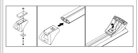
Insert the rubber buffer strip fully into the crossbar. Check the rubber buffer strip is fully inserted.
