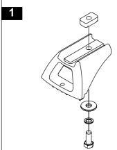
Assemble M6 x 35mm bolt, M6 spring washer, M6 square washer, adaptor block and M6 nut. Slide legs onto crossbar and finger tighten bolt.
