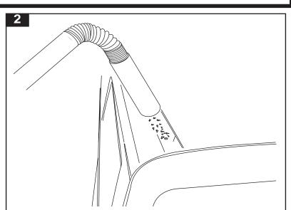
Drill approximately halfway and then use a vacuum to remove swarf from roof channel. Continue drilling
