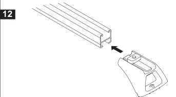
Finger tighten the Leg attachment bolt so that the Channel Nut turns to locate across the bar. The legs will require adjustment later.
