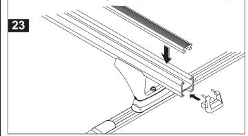
When the cross bars and legs are removed the roof pads can be covered for protection with the Mounting Pad Cover Plates.
