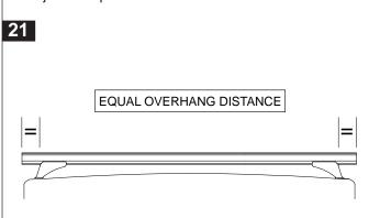
When front and rear cross bars are in required position, tension legs and cross bars.
