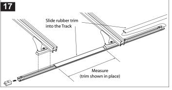
Measure and cut the rubber roof trim and put back in the vehicle roof channel at the front and rear ends of the Track. The front piece needs to be measured so the end of it sits under the windscreen rubber. The measurement and cutting of the rubber roof trim isn't critical since the End Cap will cover it. Recommend using a fine tooth hacksaw because of metal inside the rubber roof trim.
