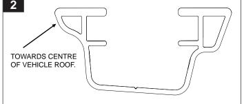
Place the track in the channel and measure from the edge of the windscreen rubber to the front of the track. The use of masking tape will help maintain this measurement while marking out holes for drilling.
