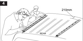
Accurately centre punch all holes before drilling.
