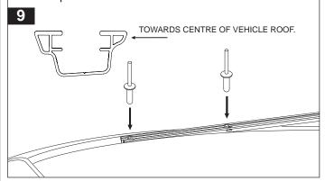
Using either a pneumatic or concertina type rivet gun, rivet the track into place. Make sure all rivets are seated firmly onto the base of the track.
