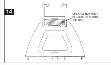
Place the Bottom Pad over the Dowel Nut Housing then Top Pad. Sit the Leg/Cross bar assembly on the Top Pad. Place the M6 Security Screw and washers through the hole in the Leg as shown and screw into the Dowel Nut. Slide Cross bar out of the way to better access the M6 Security Screw. Tightening torque is 3-4Nm. Tighten after positioning both sides equally.
