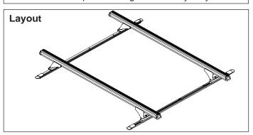
Take note of track orientation when placing in the roof channel. Both tracks are the same.
