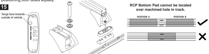
Tighten the cross bar attachment bolts. Recommended tightening torque (5Nm). Ensure that the channel nut is located across the cross bar.
