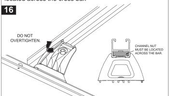
Prior to final fitment of the second cross bar/leg assembly, do a trial placement and measure the distance inbetween. Cut the rubber roof trim to this measurement. Slide the rubber roof trim into the Track as shown.
