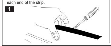
Gently lever the rubber roof trim starting with a screwdriver
