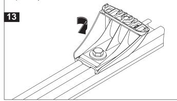
It is very important that the Channel Nut is fully located across the bar as shown.
