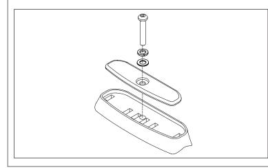
Pad cover plates are provided for when crossbars are removed.
