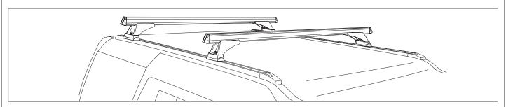
Foam pad of item 18 faces downward. Place two M6 rectangular foam backed nuts into each track. Push down on the nut and slide.
