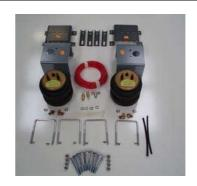
Pre fit the kit by mounting the Upper Bracket onto the spring using the 3/8" -16 flange locknuts. Attach the air fitting elbow to the airbag. Install the elbow in the air inlet hole on the top plate of the bellows. Tighten until the elbow is pointing towards the centre of the vehicle.
