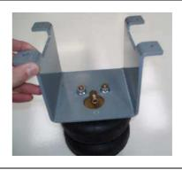
Attach the lower bracket to the airbag using the  $3/8 \times 3/4$  flange lock bolt. Next, cut the air line into two equal lengths, making the cut as square to the axis of the tubing as possible. Insert the air line into the elbow and push until a positive click is felt.
