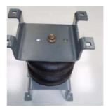
Compress the air spring assembly and place it between the leaf spring and chassis rail. Using the 3/8"-16 X 3" carriage bolts and the Bracket straps fix the lower bracket to the axle. Attach the top bracket to the framework of the vehicle directly above the bottom bracket by means of the bail clamps provided, securing with the 5/16 nuts supplied.
