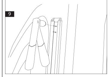
Paint cold gal over each drilled hole. This prevents the bare metal from rusting. Make sure to let the paint dry before proceeding.
