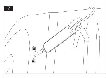
Place the track carefully onto the vehicles rooftop. Place a 5mm Rivet in each hole to allign the track. Use a Pop Rivet Gun to fix the track to the rootop. Repeat process 5 - 9 for the track on the opposite side of the vehicle.
