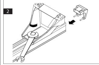
Slide the eight M6 brass hex nuts into the track as shown. Two brass nuts to each end.
