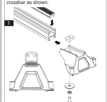
Tighten the leg to the crossbar so it can slide for adjustment. Place two end caps on each crossbar.
