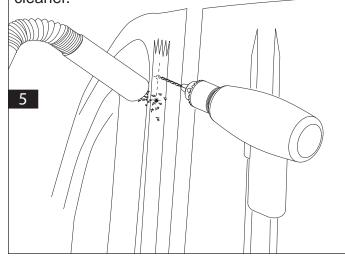
Apply Silicone or Butyl Mastic liberally over and around each drilled hole.
