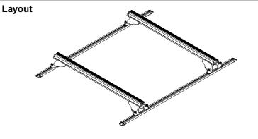
Install crossbar onto legs. Push the leg hex bolt up and turn the bolt so that the channel nut is fully located across the crossbar
