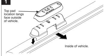
4 door Vitara: Place the pads between the round plastic covers on the roof rail at a spacing of 750mm.2 door Vitara: Place the edge of the pads 125mm from the join in the roof rail.
