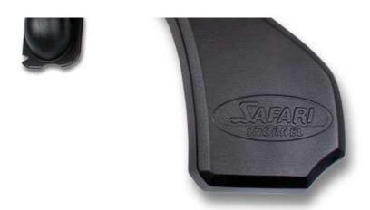
The Safari Snorkel body, air ram and inner duct are manufactured to the highest standards in durable, UV stable, cross linked polyethylene
