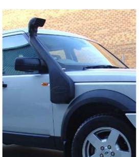
In addition, the detachable Safari air ram can be rotated to any position. This means great peace of mind for
