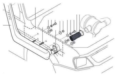
For example in order to achieve the optimum air flow and the maximum user convenience (for other under-hood accessories), a special **cuffed hose** was engineered to closely couple the snorkel body to the standard
