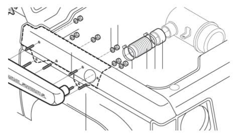
This of course applies to components that are not visible. For example a tough straight-shot hose is installed inside the inner guard and forms a positive connection to the standard air cleaner assembly.
