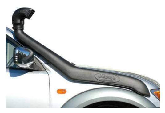
The Safari Snorkel body is manufactured to the highest standards in durable, UV stable, cross linked polyethylene material. In addition, the
