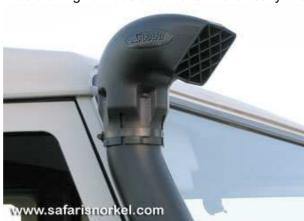
anticipated. By rotating the air ram to face away from the prevailing wind/direction of motion, the air ram delivers additional protection from the choking effects of snow build-up inside the air intake.
