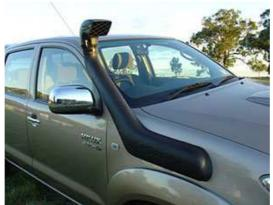
The Safari Snorkel body is manufactured to the highest standards in durable, UV stable, cross linked polyethylene material. In addition, the substantial material wall thickness delivers huge physical strength to ensure that the snorkel breezes through the toughest offroad conditions on the planet.
