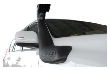
The genuine Safari Snorkel body and air ram is manufactured to the highest standards in durable, UV stable, cross linked polyethylene material. In addition, the substantial material wall thickness delivers huge physical strength to ensure that the snorkel breezes through the toughest off-road conditions on the planet.
