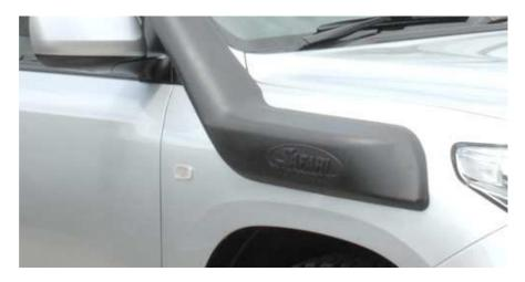
Close attention to the internal cross sectional profile and area, air velocity and flow path through each and every point along the entire length of the snorkel system ensures that the greatest air flow is achieved. The result is maximum engine performance and the best possible fuel economy.
