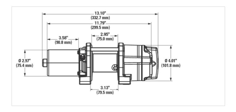
Winch Dimensions: 13.1" L. x 4.53" D. x 4.69" H. (333mm L. x 115mm D. x 119mm H.)
