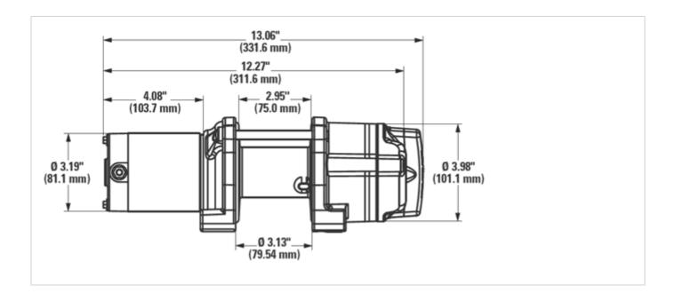
Winch Dimensions: 13.1" L. x 4.53" D. x 4.69" H. (333mm L. x 115mm D. x 119mm H.)
