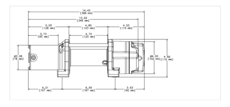
Winch Dimensions: 14.78" L. x 4.53" D. x 4.69" H. (375mm L. x 115mm D. x 119mm H.)
