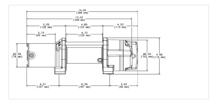
Winch Dimensions: 14.42" L. x 4.53" D. x 4.69" H. (375mm L. x 115mm D. x 119mm H.)
