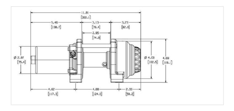
Winch Dimensions: 11.81" L. x 4.53" D. x 4.69" H. (300mm L. x 115mm D. x 119mm H.)
