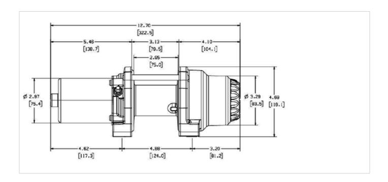
Winch Dimensions: 12.7" L. x 4.53" D. x 4.69" H. (323mm L. x 115mm D. x 119mm H.)
