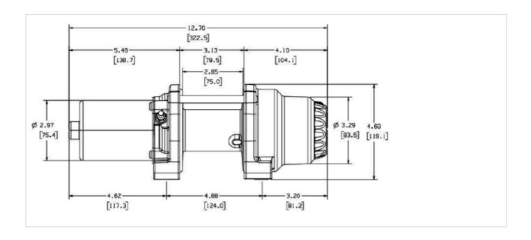
Winch Dimensions: 12.7" L. x 4.53" D. x 4.69" H. (323mm L. x 115mm D. x 119mm H.)
