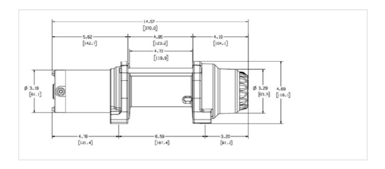
Winch Dimensions: 14.57" L. x 4.53" D. x 4.69" H. (370mm L. x 115mm D. x 119mm H.)
